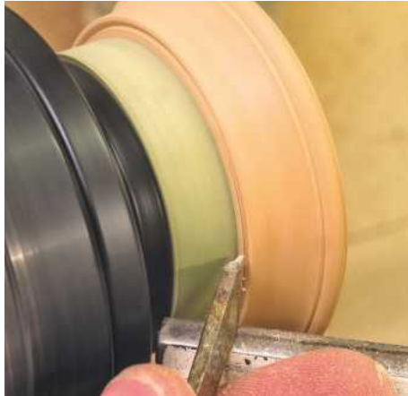
▲ Pic.20 Set the toolrest around the back and make a cut around 45° into the base; this should be around 2mm deep to accept the baize
